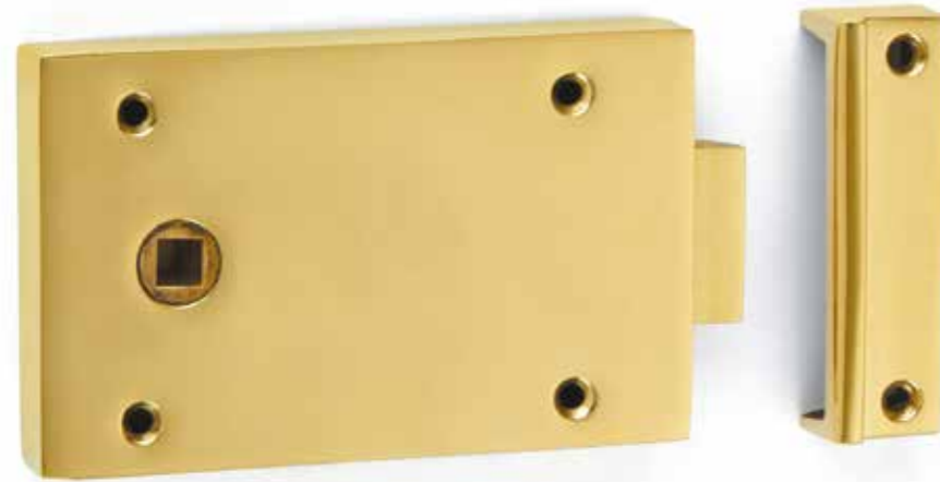
1871 Rim Lock This item is handed (Right Hand shown) These locks are 2 lever and supplied with 2 keys. 127mm (5"), 152mm (6"), 177mm (7") or 203mm (8")
