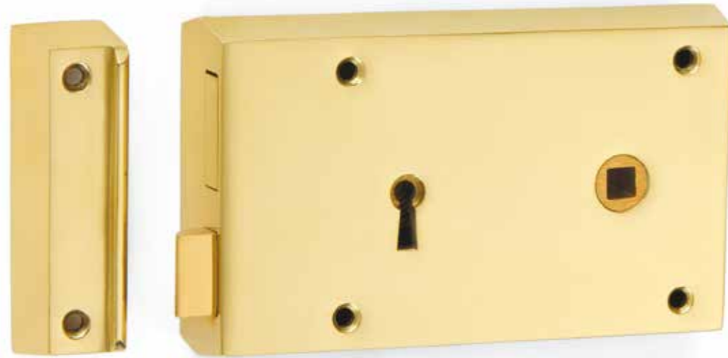
1871 Rim Lock This item is handed (Right Hand shown) These locks are 2 lever and supplied with 2 keys. 127mm (5"), 152mm (6"), 177mm (7") or 203mm (8")
