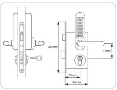
Model 520/525 With full 'Panic Function' mortice lock & cylinder
