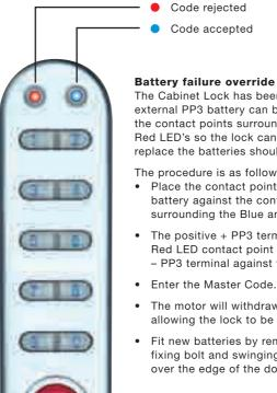
The Cabinet Lock has been designed so an external PP3 battery can be placed against the contact points surrounding the Blue and Red LED's so the lock can be opened to replace the batteries should they fail.
