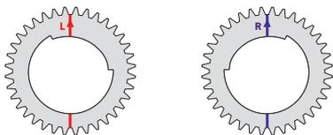
Flip over the spindle hub so that it shows a red line and the letter L. Ensure that the red lines are aligned and vertical.
