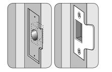
**NB** The plunger beside the latchbolt deadlocks the latchbolt and protects it against manipulation.
