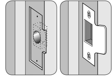
**NB** The plunger beside the latchbolt deadlocks the latchbolt and protects it against manipulation. IT MUST NOT enter the strike plate aperture when the door is closed.
