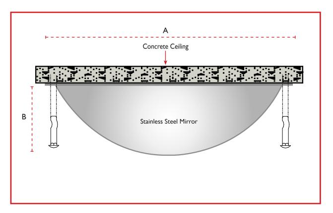
NOTE: Domes with Counter-Sunk Holes can be ligature free when mounted directly to the ceiling with appropriate tamperproof fixings.
