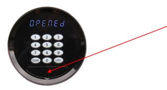
Initially the keypad may not have batteries fitted. To insert batteries pull the door open, remove the grey cover from inside the drawer and load 4pcs 1.5V AA Alkaline batteries. Replace the battery cover.
