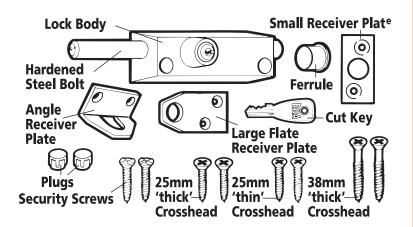
Close the door and position unlocked Multi Purpose Bolt on the door. Gently tap bolt end to mark position on fixed frame. Drill an 1mm hole in fixed frame. With bolt in locked position locate lock body as high as possible on frame whilst allowing free movement of the door when unlocked. Ensuring that the bolt sits at least to the depth of groove in to drilled hole (when locked), mark screw hole positions.
